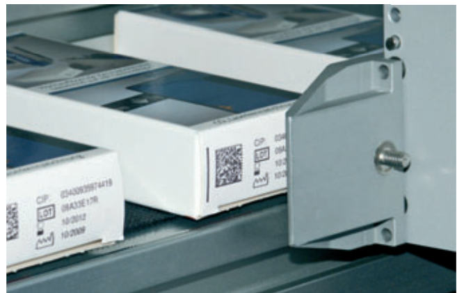
Cardboard box coding using DataMatrix Code
